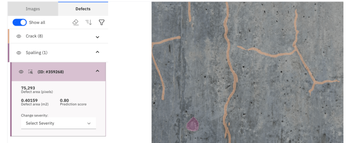
Fig. 3. Visualization of defects in specific image with associated confidence score as computed by the AI-model.
