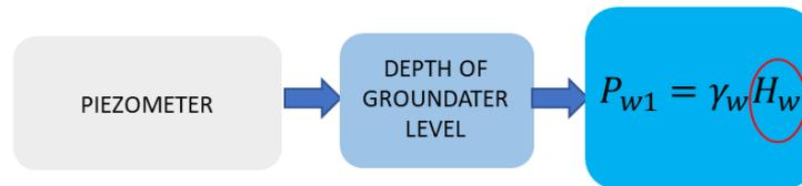
Figure 8.28 – Use of data for hydraulic actions-piezometers
