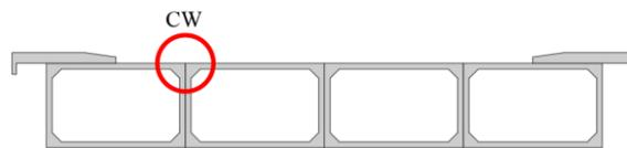
Figure 2.8 – Conceptual weaknesses in a precast multicellular cross section (Extract from [4])
